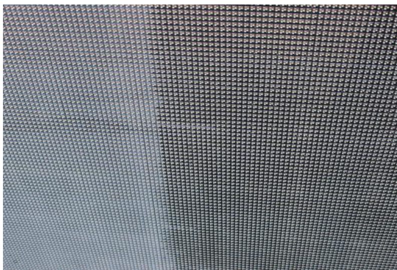
LED's and shades covered with dirt
